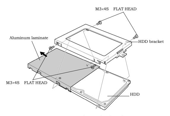
Figure 4-5 Removing the HDD bracket and HDD
